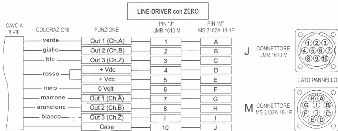
Fig. 4.14 Connections of the encoder.
