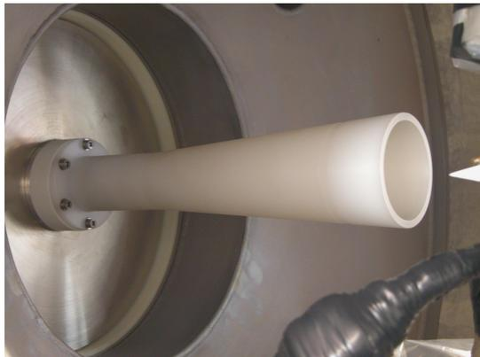
Fig. 8.2: Nozzle mounted at the exit of the settling chamber.
