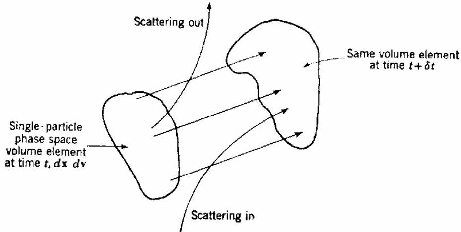
**Figure 1.1** - Schematic representation of the motion of an infinitesimal volume element in single-particle phase space volume.
