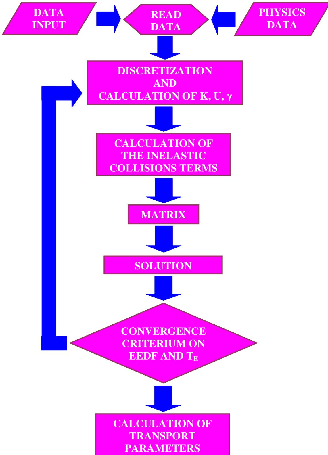
*Figure 1.3 - Flux diagram of the numerical code solving the Boltzmann equation.*
