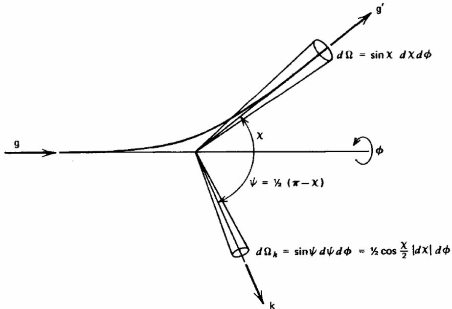
*Figure 1.2 - Schematic representation of the collision plane.*
