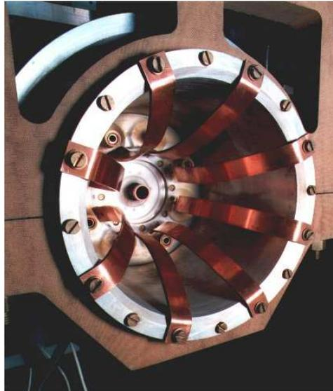
*Figure 2.2 – Picture of the MPD thruster.*
