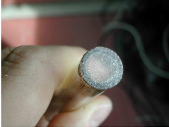
*Figure 2.12 - Picture of the coat formed on the probe.*
