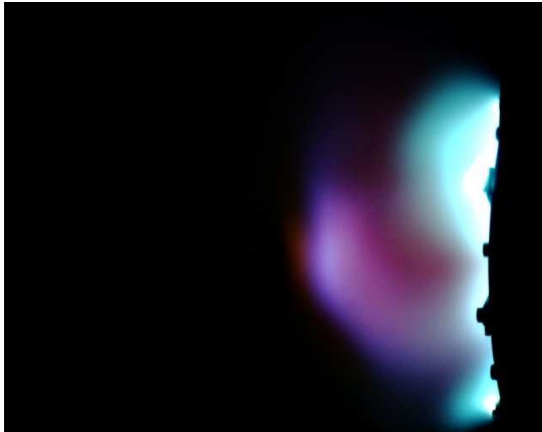
Figure 4.3 – Image of the plasma plume recorded with t_{\text{exp}} = 6 \mu\text{s} and t_d = 50 \mu\text{s} .
