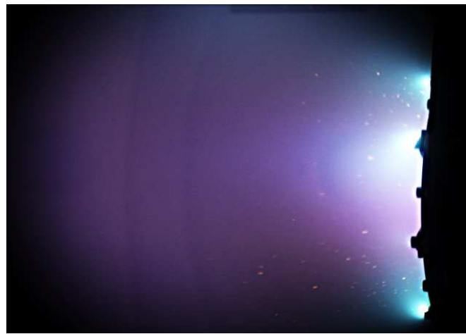
Figure 4.4 - Plasma plume in regime conditions recorded with t_{exp} = 5 \mu s and t_d = 1 ms .
