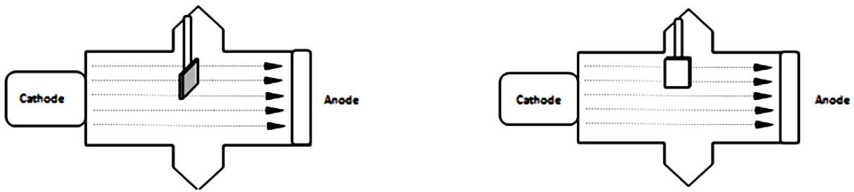
Figure 7.4 Langmuir probe parallel (left)/perpendicular(right) configuration with/on field lines
