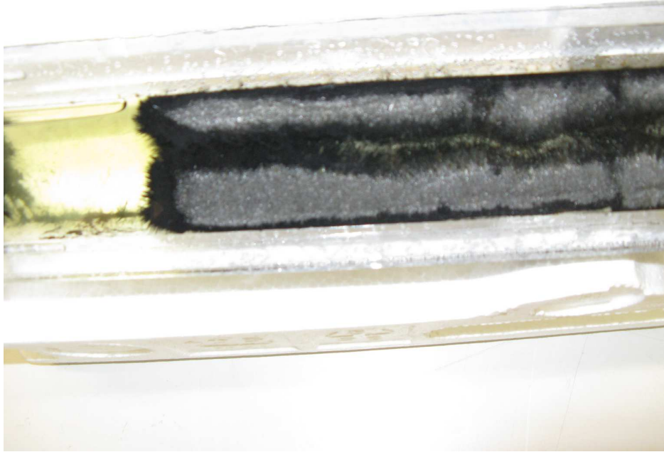
Figure 3.5: Picture of a filter packaged in the wrong way: a channel through which the flow is facilitated is visible.
