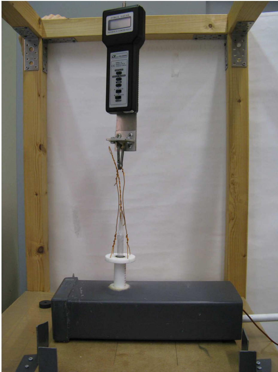
Figure A.1: Experimental set-up able to measure the magnetic force exerted on a sample.
