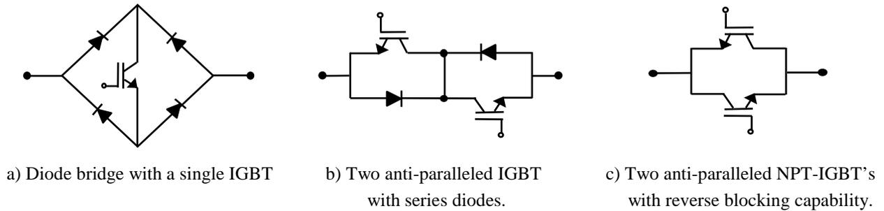
Fig.3.1 Possible discrete implementations of a bi-directional switch.
