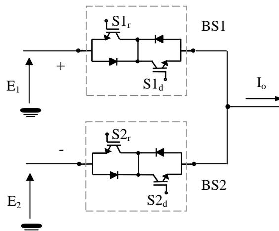
Fig.3.5 General commutation circuit of two bi-directional switches.
