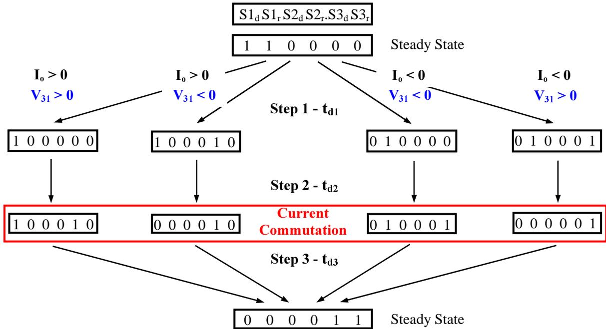
Fig.3.13 Three-step switching diagram based on output current and input voltage sign detection. BS1  $\rightarrow$  BS3 case.  $V_{31} = E_3 - E_1$  is the line-to-line commutation voltage.  $I_o$  is the output current.
