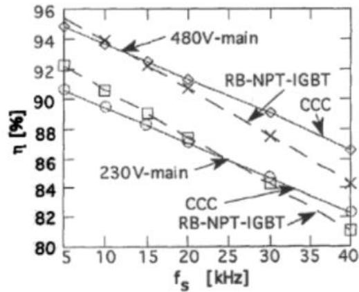
Fig.3.3 Simulated matrix converter efficiency. (reprinted from [8], pp. 111).
