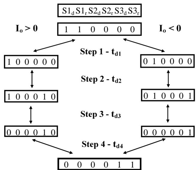
Fig.3.7 Switching diagram for three bi-directional switches.
