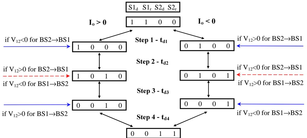
Fig.3.6 Four-step switching diagram for two bi-directional switches.
