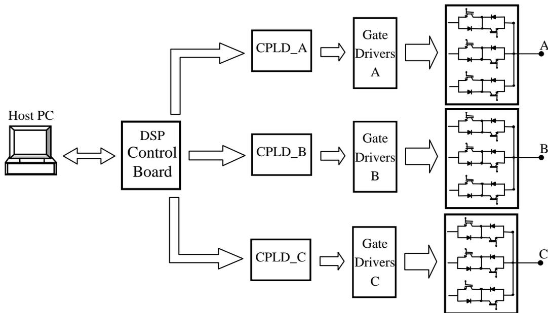
Fig.3.15 Block diagram of matrix converter control system.
