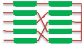
Fig 11.2 Five-phase machines connection
