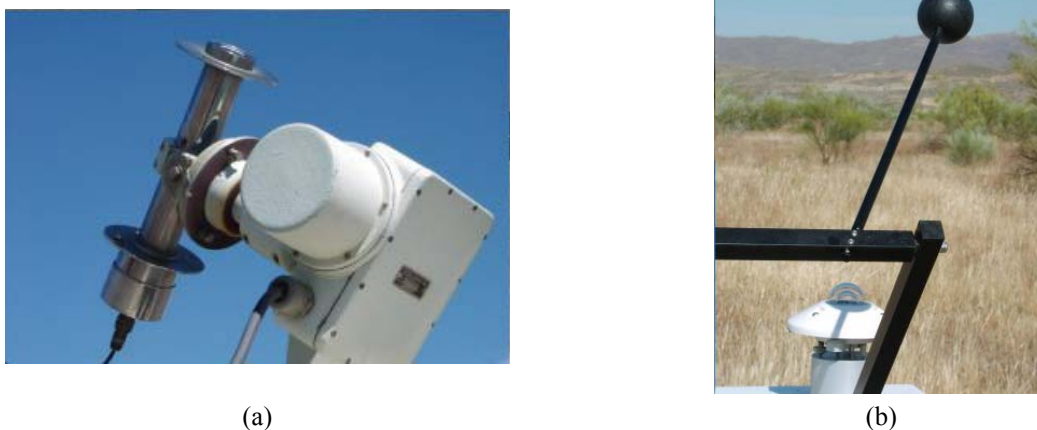
Fig. 12. Irradiance sensors (a) two-axis tracked pyrliometer for direct normal irradiance measurements (b) with shading ball for diffuse irradiance measurements.
