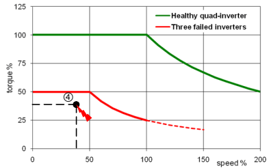
Fig. 6.8: Considered operating points in torque-speed diagram for healthy (4 VSIs) and three failed inverter (1 VSIs) conditions.
