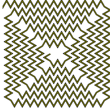
Figure B.0.4.: Planar zig-zag spiral inductor with its axis.
