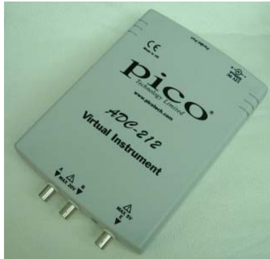
Figure 5-9. Acquisition and Analog to Digital conversion board.
