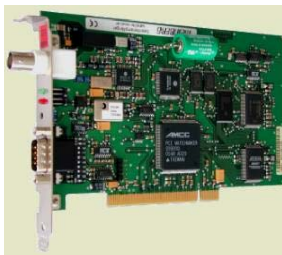
Figure 5-6. The antenna of the GPS station. Figure 5-7. The PCI board of the GPS system.
