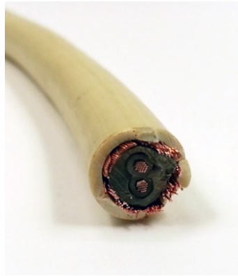
Figure 3.3. LOCA measurement/instrumentation cable. EVA-based insulation.
