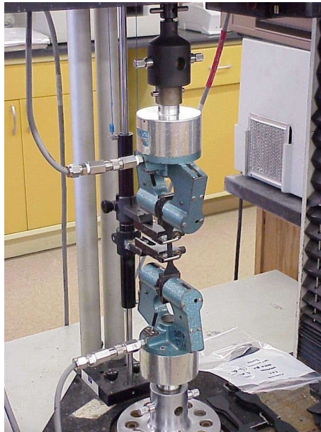
Figure 2.1. Tensile testing machine for rubbers.
