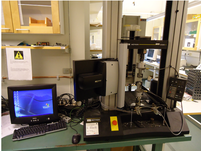
Figure 3.10. Tensile testing experimental setup.
