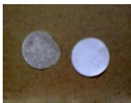
Figure 5.22 Electrospun separator after (left) and before (right) being pressed.
