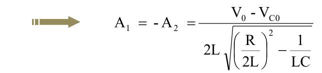
Transient solution in case A – Overdamped case :  $\alpha > \omega_0$ , R >  $2\sqrt{L/C}$
