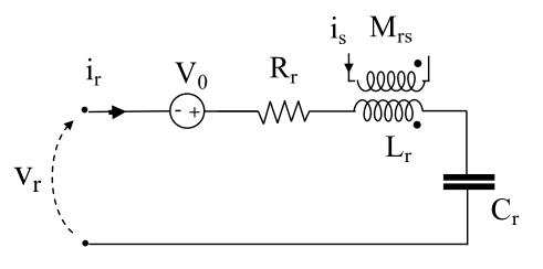
$$v_{r}(t) = L_{r} \frac{di_{r}}{dt} + M_{rs} \frac{di_{s}}{dt} + \frac{1}{C_{r}} \int_{-\infty}^{t} i(t')dt' + R_{r}i_{r}(t) - V_{0}$$
