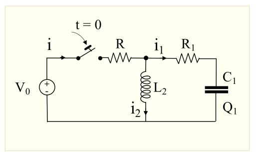
$$\begin{cases} L_2 \frac{d i_2}{d t} + R i - V_0 = 0 \\ \frac{Q_1}{C_1} + \frac{1}{C_1} \int_0^t i_1(t') dt' + R_1 i_1 + R i - V_0 = 0 \\ i - i_1 - i_2 = 0 \end{cases}$$
