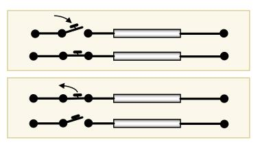
On-off or off-on mode changes of switches or sudden changes of the excitation (voltage or current source modeled as step functions) are the cause of transients followed by a steady state operation that is the response of the circuit to the changed condition.
