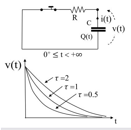
The RC circuit can be obtained as an equivalent circuit (Thévenin/Norton).
