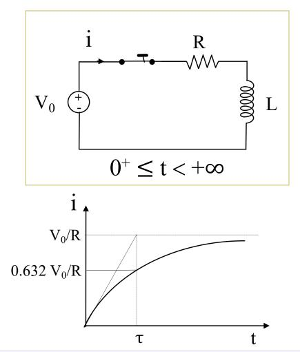
The <u>complete response</u> of the RL circuit is the steady-state response (forced response)  $[i(+\infty) = 0]$  added to the transient response (<u>natural response</u>).
