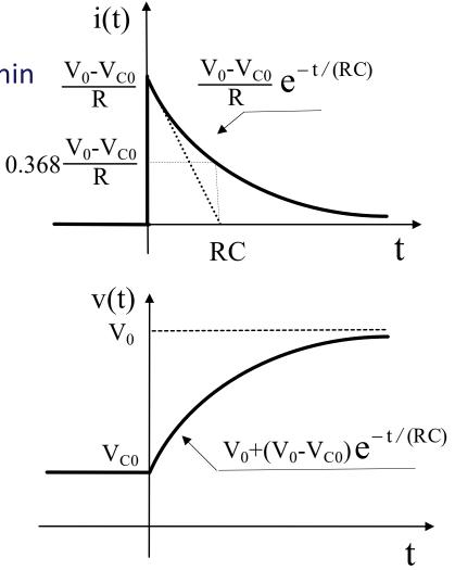
The analysis of the regime at  $t = +\infty$  gives the steady-state response (forced response)  $[i(+\infty) = 0, v(+\infty) = V_0]$  that added to the transient response (natural response) gives the complete response of the RC circuit suddenly excited.
