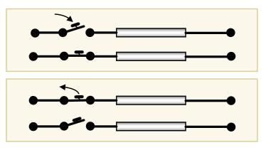
The storage elements may change their operation state with fulfilling the *energy conservation principle*. As a consequence of it storage elements prevent instantaneous variation of energy in the transit from  $t = 0^-$  to  $t = 0^+$ :
