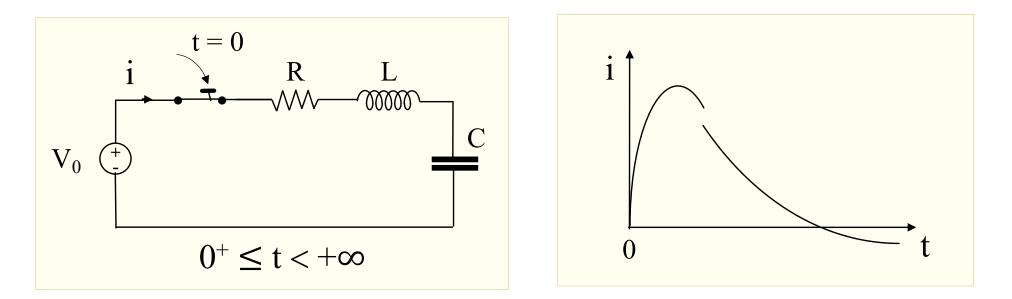
**Case B**- *critically damped case*:  $\alpha = \omega_{0} \rightarrow R = 2 \sqrt{L/C}$ ;  $x_{1}$ ,  $x_{2}$  negative coincident solutions
