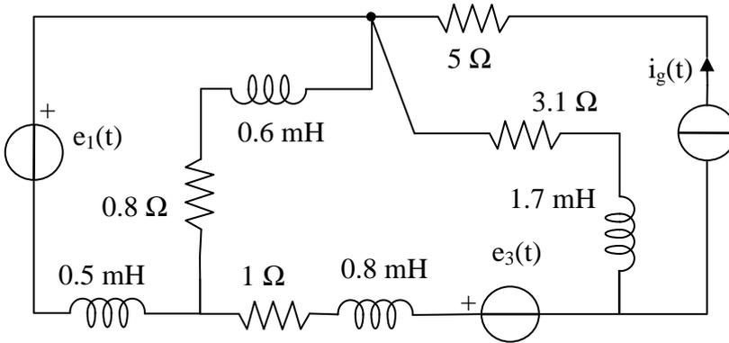
$$e_1(t) = \sqrt{2} 15 \cos(\omega t) \text{ V}, \quad e_3(t) = \sqrt{2} 8 \cos(\omega t) \text{ V}, \quad \omega = 1000 \text{ rad/s}$$
