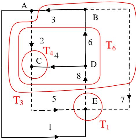
$$\begin{array}{l} \text{LKC}_{T_1} \\ \text{def.} \\ \text{LKC}_{T_3} \\ \text{LKC}_{T_4} \\ \text{def.} \\ \text{LKC}_{T_6} \\ \text{def.} \\ \text{def.} \end{array} \left\{ \begin{array}{l} i_1 = -i_{c_2} - i_{c_3} + i_{c_4} \\ i_2 = i_{c_1} \\ i_3 = i_{c_1} - i_{c_2} - i_{c_3} + i_{c_4} \\ i_4 = -i_{c_1} + i_{c_2} \\ i_5 = i_{c_2} \\ i_6 = i_{c_1} - i_{c_2} + i_{c_4} \\ i_7 = i_{c_3} \\ i_8 = i_{c_4} \end{array} \right.$$
