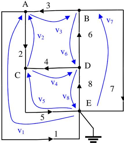
$$\begin{array}{l} \text{LKT(1)} \\ \text{LKT(2)} \\ \text{LKT(3)} \\ \text{LKT(4)} \\ \text{LKT(5)} \\ \text{LKT(6)} \\ \text{LKT(7)} \\ \text{LKT(8)} \end{array} \left\{ \begin{array}{l} v_1 = e_A \\ v_2 = e_A - e_C \\ v_3 = e_B - e_A \\ v_4 = e_D - e_C \\ v_5 = e_C \\ v_6 = e_D - e_B \\ v_7 = e_B \\ v_8 = -e_D \end{array} \right.$$
