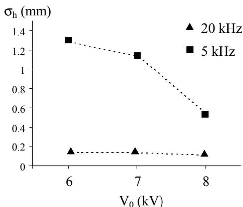
Fig.2. - Standard deviation of the meniscus height on the symmetry axis.
