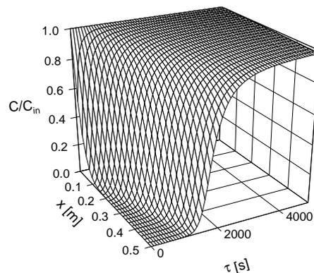
Fig. 9.a. - Loading of a magnetic filter: the time behaviour of the ratio between the particle concentration in the fluid  $C$  and the inlet particle concentration  $C_i$  along the axis of the filter is shown.
