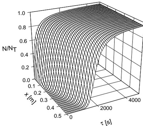
Fig. 9.b. - Loading of a magnetic filter: the ratio between the captured particle concentration  $N$  and the saturation value  $N_T$  for the captured particle concentration is shown.
