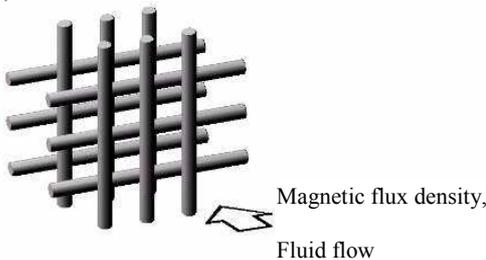
Fig. 7. - Schematic view of a matrix in a HGMS.
