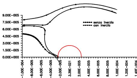
Fig. 8.a. - Trajectories for paramagnetic particles.
