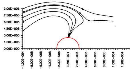
Fig. 8.b. - Trajectories for diamagnetic particles.
