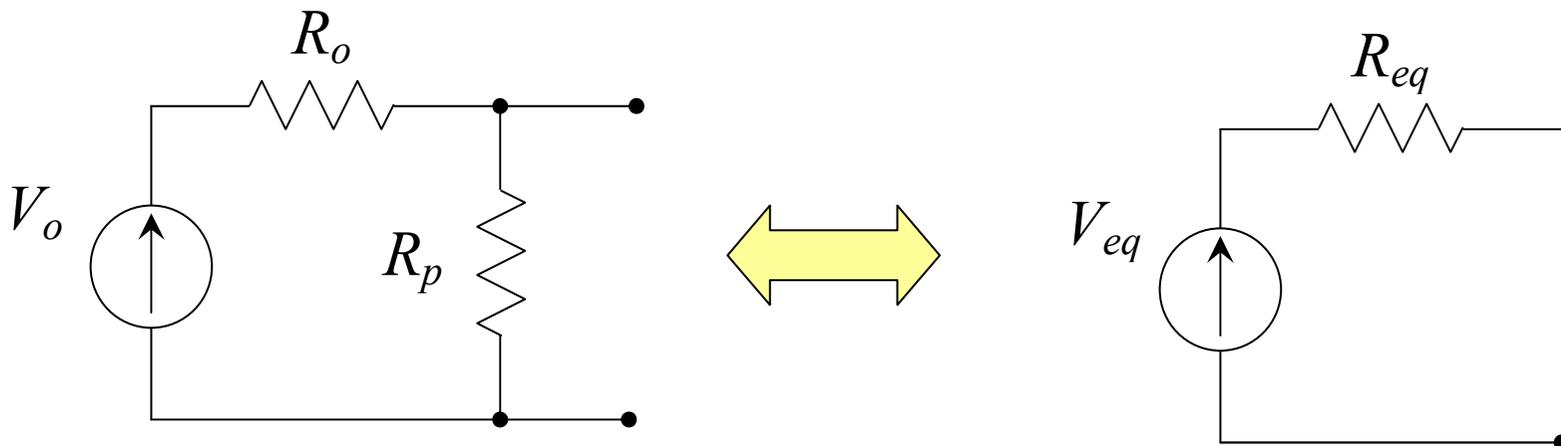
$$\left\{ \begin{array}{l} V_{eq} = \frac{V_o}{R_o + R_p} R_p \\ R_{eq} = \frac{R_o R_p}{R_o + R_p} \end{array} \right.$$
