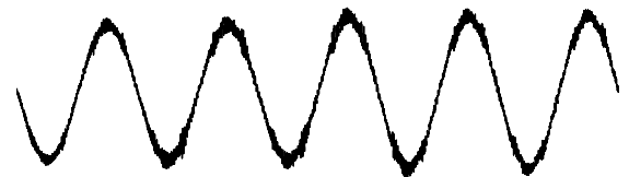
Fig. 10. Phase voltage and current applied to the primary winding of the transformer by the dual two-level converter.
