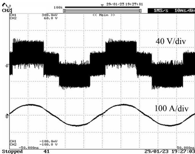
Fig. 13. Output phase voltage (over 5 levels) and current.
