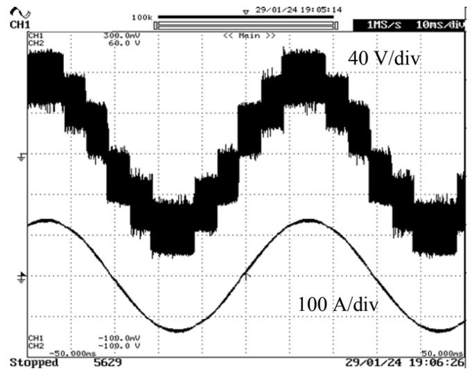
Fig. 14. Output phase voltage (over 9 levels) and current.
