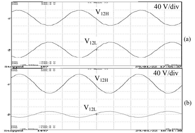
Fig. 12. Averaged line-to-line output voltages (a)  $m=1/2$ ,  $k=1/2$  (balanced); (b)  $m=1/2$ ,  $k=3/4$  (unbalanced).
