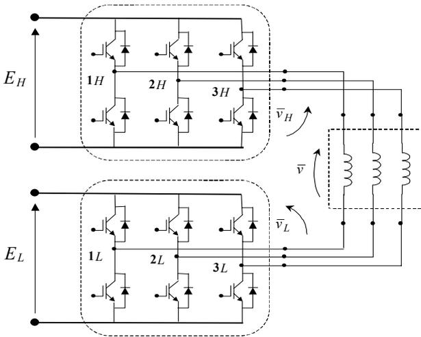
Fig. 3. Electric scheme of the multilevel converter.
