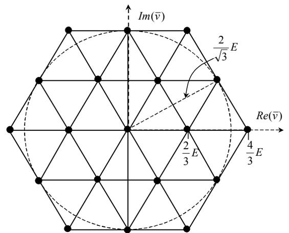
Fig. 4. Output voltage vectors of the multilevel converter.
