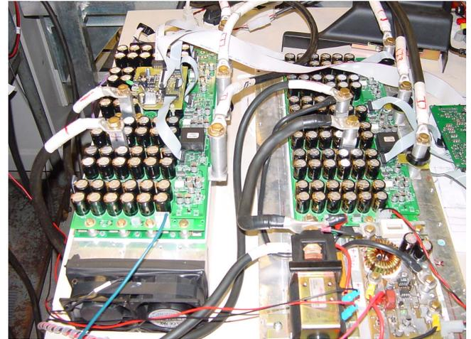
Fig. 10. Picture of the power stage of the full scale converter.
