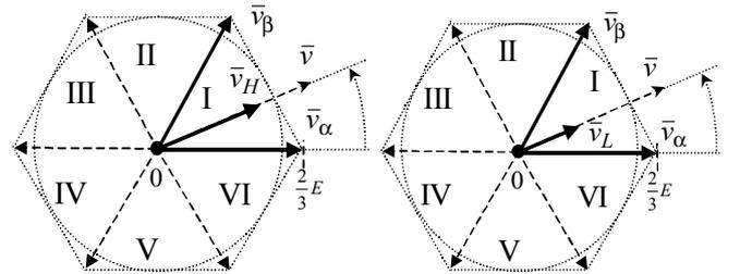
Fig. 6. Voltage vectors  $\bar{v}_H$  and  $\bar{v}_L$  generated by using the same two adjacent active vectors  $\bar{v}_\alpha, \bar{v}_\beta$ .
