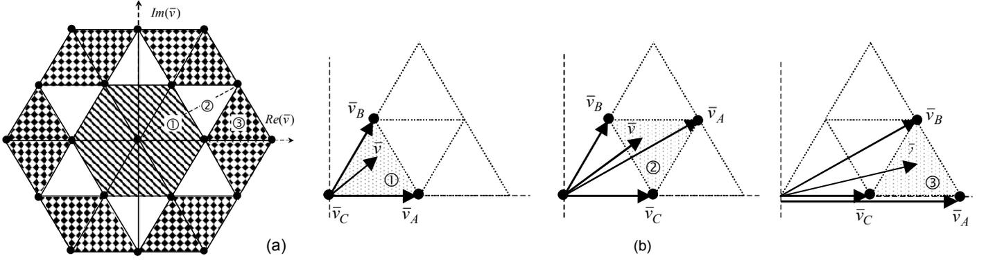
Fig. 5. (a) Highlight of the triangles in the three different regions ①, ②, and ③; (b) Vector composition to obtain the output voltage in the three different regions.
