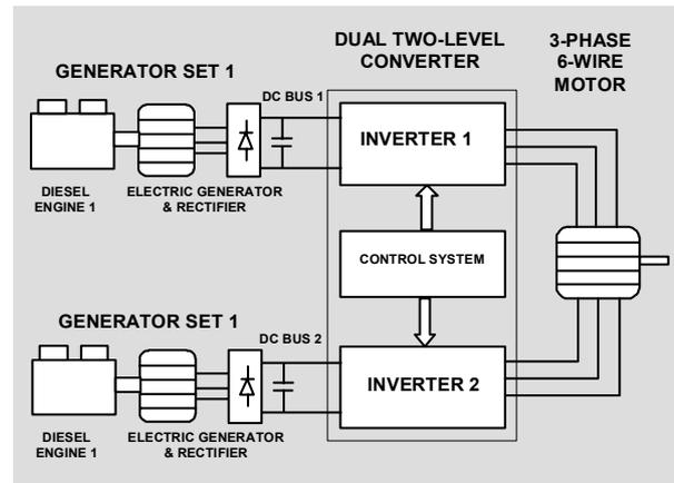
Fig. 2. Basic scheme of the diesel-electric propulsion system.
