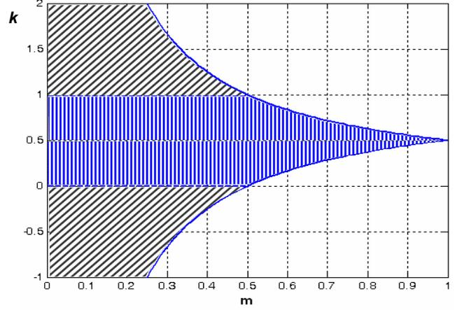
Fig. 7. Limits of the power ratio  $k$  vs. the modulation index  $m$ .
