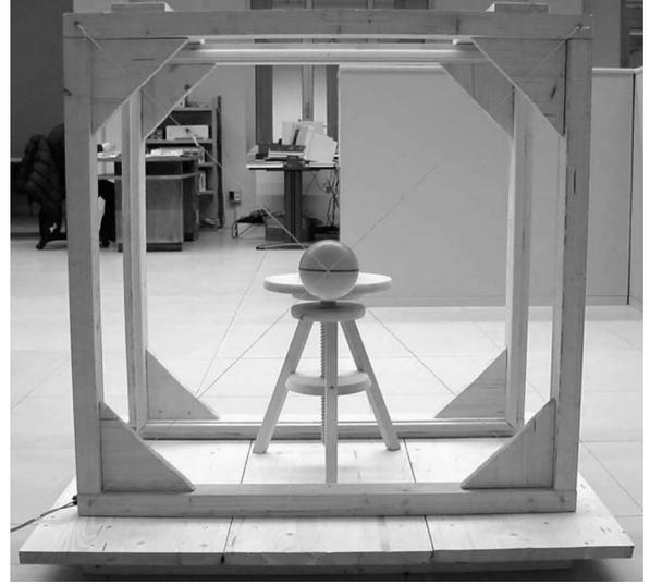
Fig. 3. Photograph of the Helmholtz coil realized by a wood structure. The magnetic sensor is placed at the center of one of the two square coaxial loops.
