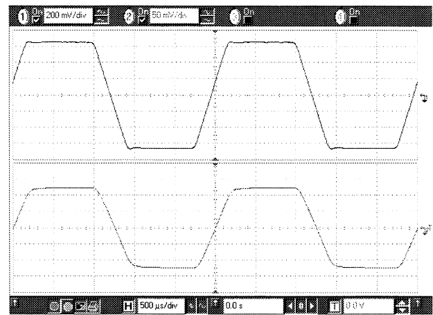
Fig. 6. Trapezoidal field waveform (400 Hz)
