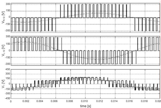
Fig. 15 Dual two-level converter voltage for  $m = 1/2, k = 1/3$
