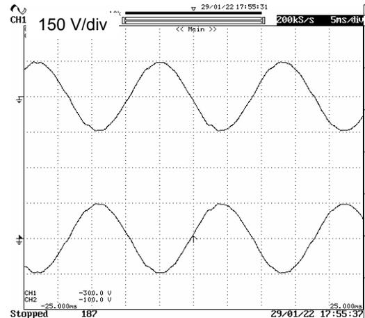
Fig. 19. Filtered line to line voltage generated by the dual two-level converter at the right side (top) and at the left side (bottom),  $m=1/2$ ,  $k = 1/2$  (balanced)
