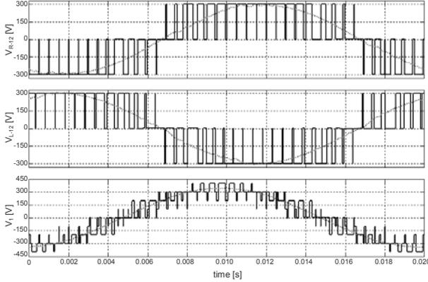
Fig. 13 Dual two-level converter voltage for  $m = 1, k = 1/2$
