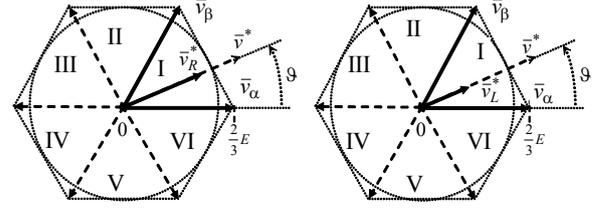
Fig. 4. Reference voltage vectors  $\bar{v}_R$  and  $\bar{v}_L$  generated by using the same two adjacent active vectors  $\bar{v}_\alpha, \bar{v}_\beta$ .
