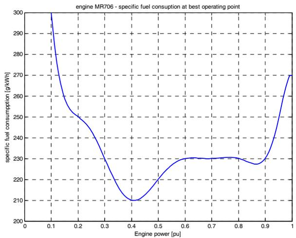
Fig. 7. Engine MR706 Specific fuel consumption at the best operating point
