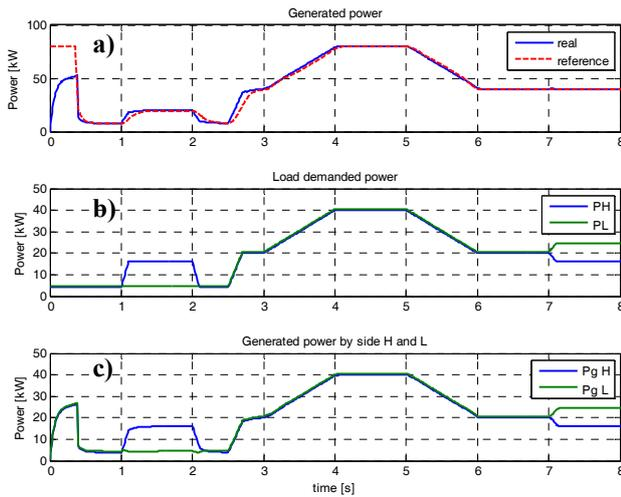
Fig. 10. Power. a) generated by the generation system; b) demanded by output drive R and L; c) supplied to drive R and L
