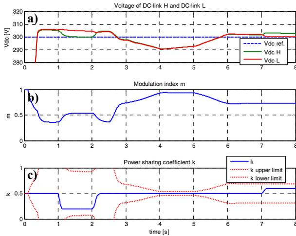
Fig. 11. a) dc-link voltage, b) modulation index, c) power sharing coefficient
