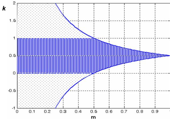
Fig. 5. Limits of power sharing coefficient  $k$  vs. modulation index  $m$ .
