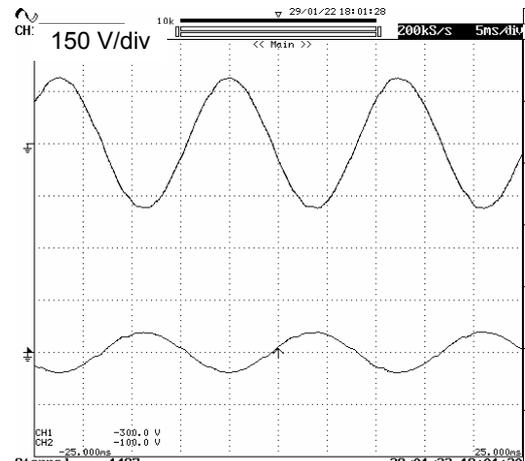
Fig. 20. Filtered line to line voltage generated by the dual two-level converter at the right (top) side and at the left (bottom) side,  $m=1/2$ ,  $k = 3/4$  (unbalanced)
