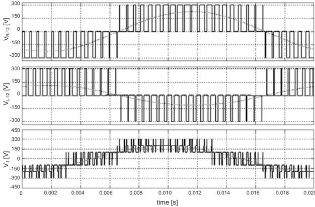
Fig. 14 Dual two-level converter voltage for  $m = 1/3, k = 2/3$
