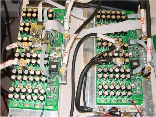
Fig. 16. Picture of the dual two level inverter prototype.
