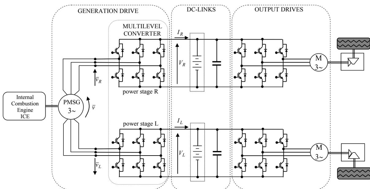
Fig. 1. Electric scheme of the series hybrid transmission
