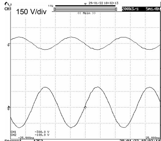
Fig. 21. Filtered line to line voltage generated by the dual two-level converter at the right (top) side and at the left (bottom) side,  $m=1/2$ ,  $k = 1/4$  (unbalanced)
