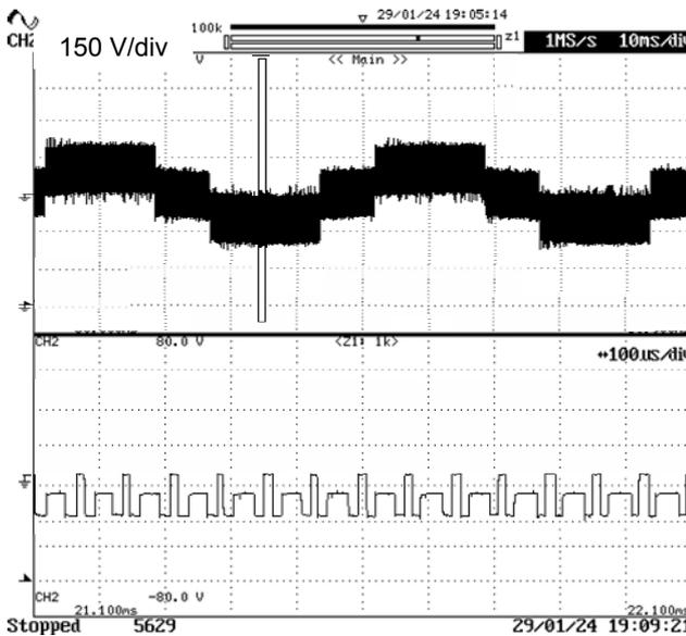
Fig. 18. Phase voltage applied to the PMSG by the dual two-level converter for  $m = 1/2$ ,  $k = 2/3$
