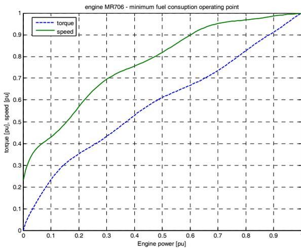
Fig. 6. Engine MR706, torque and speed operating points vs. power at minimum fuel consumption
