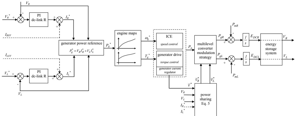
Fig. 2. High level control algorithm of the series hybrid system
