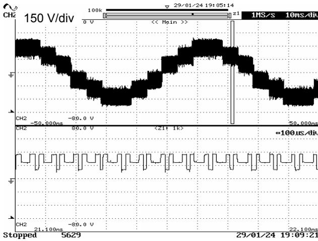
Fig. 17. Phase voltage applied to the PMSG by the dual two-level converter for  $m = 1$ ,  $k = 1/2$
