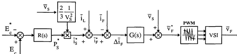
Fig. 2. Block diagram of the control system.
