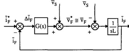
Fig. 4. Block diagram of the AC current control loop.
