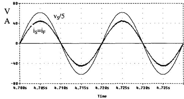
Fig. 8.4. Source current and source voltage waveforms in steady-state operating conditions after the load switching-off.
