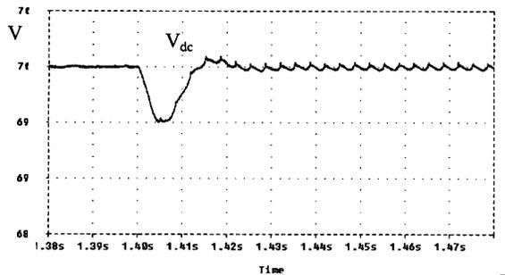
Fig.9.1. DC-link voltage variation during the load switching-on.
