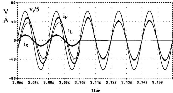
Fig. 8.3. Current and source voltage waveforms during the load switching-off.
