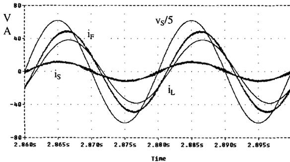
Fig. 7.4. Current and source voltage waveforms in steady-state operating conditions after the load switching-on.
