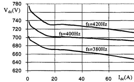
Fig. 6. Compensating effect of the series capacitance for different angular frequency values.
