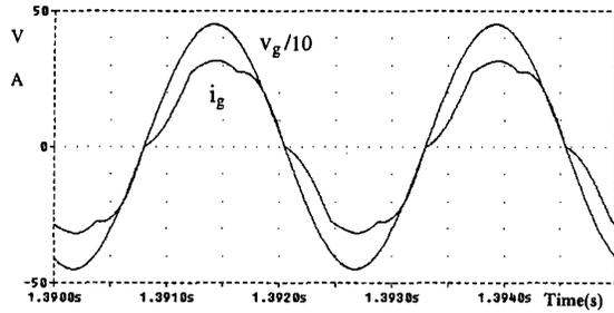
Fig. 5. Phase current and scaled phase voltage waveforms at rated speed.
