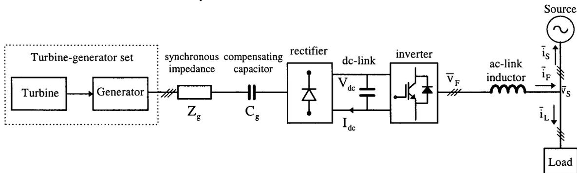
Fig. 1. Block diagram of the cogeneration system.
