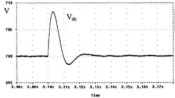
Fig. 8.2. DC-link voltage variation during the load switching-off.
