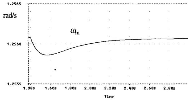
Fig. 7.1. Turbine speed variation during the load switching-on.
