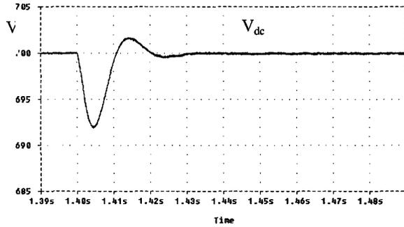
Fig. 7.2. DC-link voltage variation during the load switching-on.
