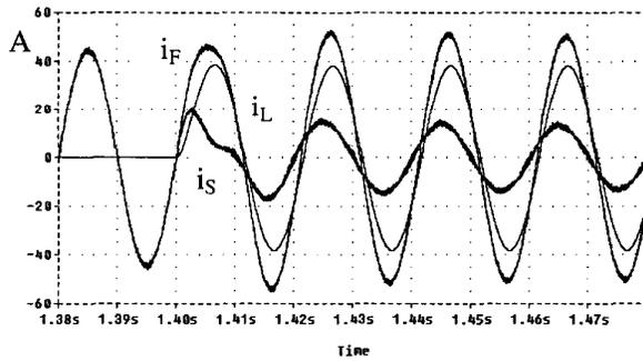
Fig. 7.3. Current waveforms during the load switching-on.
