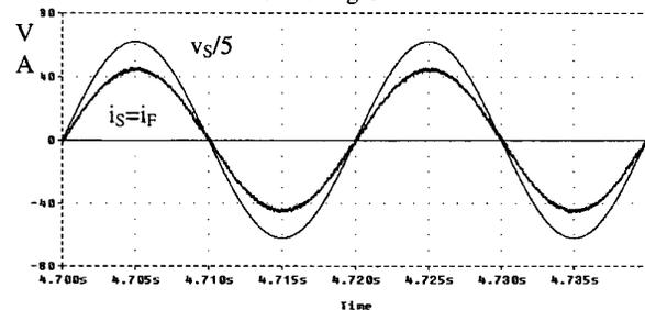
Fig.10.3. Source current and source voltage waveforms in steady-state operating conditions after the load switching-off.
