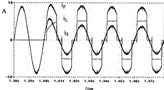
Fig.9.2. Current waveforms during the load switching-on.
