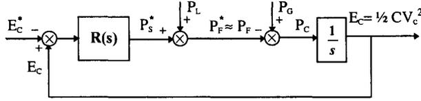
Fig. 3. Block diagram of the DC-link voltage control loop.
