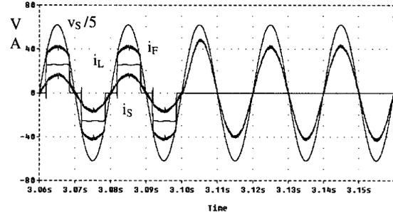
Fig.10.2. Current and source voltage waveforms during the load switching-off.
