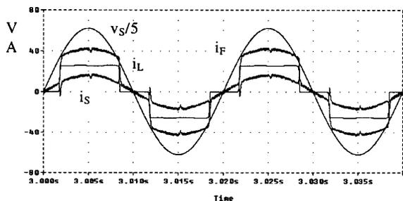
Fig.9.3. Current and source voltage waveforms in steady-state operating conditions after the load switching-on.
