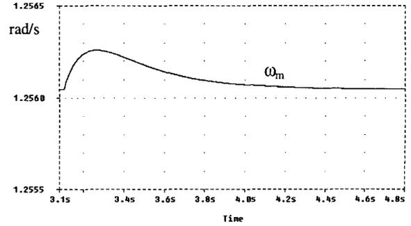
Fig. 8.1. Turbine speed variation during the load switching-off.
