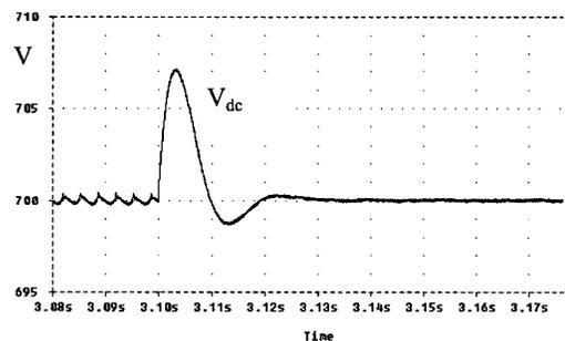
Fig.10.1. DC-link voltage variation during the load switching-off.
