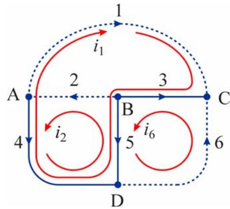
**Maglia 1:**  $(R_1 + R_3 + R_4 + R_5)i_1 - (R_4 + R_5)i_2 + (R_3 + R_5)i_6 = v_{G3}$
