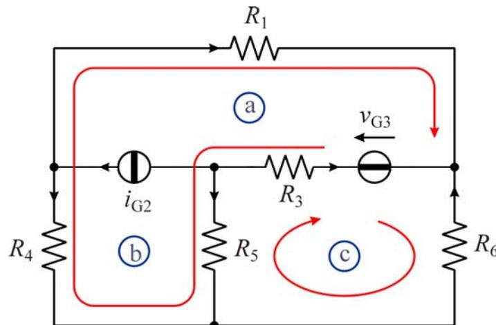
**Superanello a-b:**  $(R_1 + R_3)i_a + (R_4 + R_5)i_b - (R_3 + R_6)i_c = v_{G3}$
