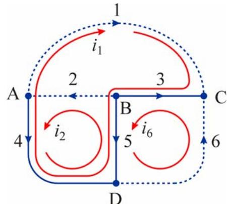
**M. 1:**  $(R_1 + R_3 + R_4 + R_5)i_1 - (R_4 + R_5)i_2 + (R_3 + R_5)i_6 = v_{G3}$
