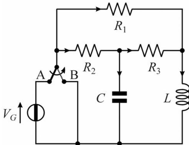
$$\begin{aligned} R_1 &= 4 \Omega \\ R_2 &= 2 \Omega \\ R_3 &= 2 \Omega \\ C &= 0.5 \text{ F} \\ L &= 0.5 \text{ H} \\ V_G &= 12 \text{ V} \end{aligned}$$
