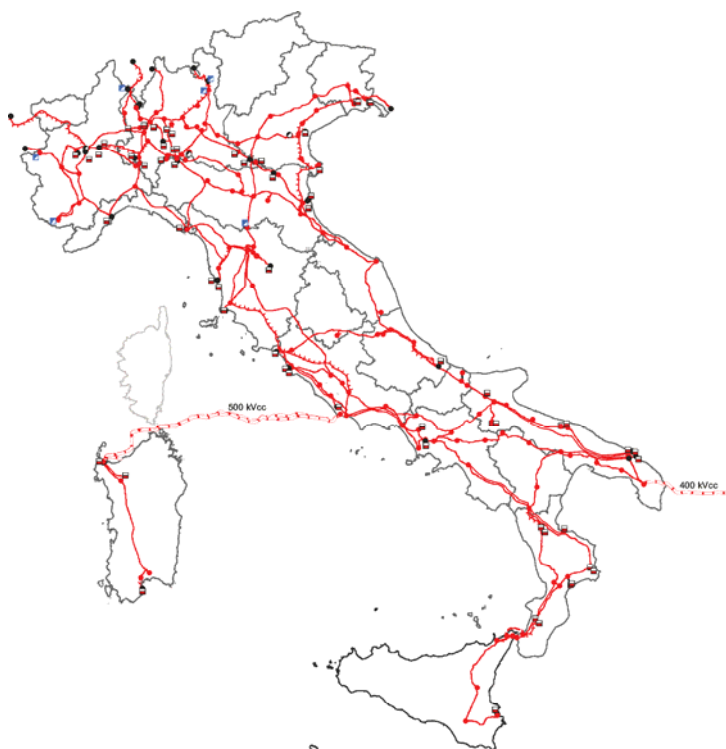
Rete a 380 kV (31-12-2017)
