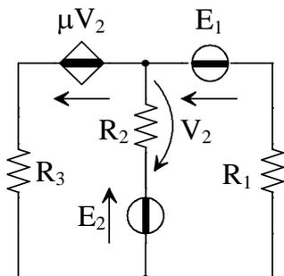
$$\begin{aligned} R_1 &= 4 \, \Omega \\ R_2 &= 1 \, \Omega \\ R_3 &= 2 \, \Omega \\ E_1 &= 30 \, \text{V} \\ E_2 &= 12 \, \text{V} \\ \mu &= 3 \end{aligned}$$
