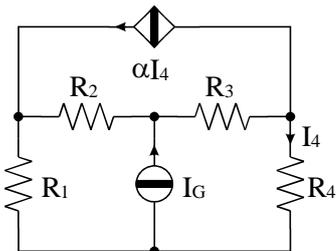
$$\begin{aligned} R_1 &= 2 \, \Omega \\ R_2 &= 1 \, \Omega \\ R_3 &= 4 \, \Omega \\ R_4 &= 2 \, \Omega \\ I_G &= 8 \, \text{A} \\ \alpha &= 3 \end{aligned}$$
