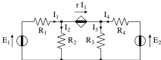
$$\begin{aligned} R_1 &= 6 \Omega \\ R_2 &= 6 \Omega \\ R_3 &= 6 \Omega \\ R_4 &= 6 \Omega \\ E_1 &= 24 \text{ V} \\ E_2 &= 24 \text{ V} \\ r &= 4 \Omega \end{aligned}$$
