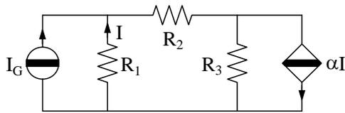
$$\begin{aligned} R_1 &= 5 \, \Omega \\ R_2 &= 1 \, \Omega \\ R_3 &= 2 \, \Omega \\ I_G &= 2 \, \text{A} \\ \alpha &= 3 \end{aligned}$$
