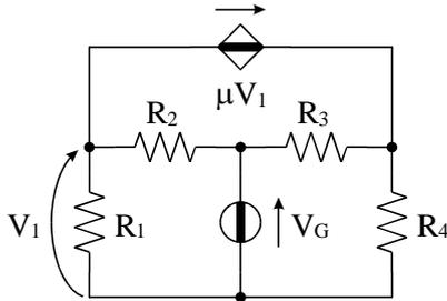
$$\begin{aligned} R_1 &= 3 \Omega \\ R_2 &= 1 \Omega \\ R_3 &= 2 \Omega \\ R_4 &= 6 \Omega \\ V_G &= 16 \text{ V} \\ \mu &= 3 \end{aligned}$$
