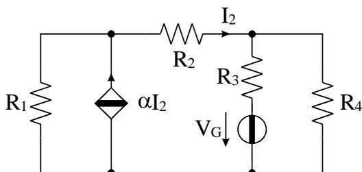
$$\begin{aligned} R_1 &= 3 \, \Omega \\ R_2 &= 3 \, \Omega \\ R_3 &= 6 \, \Omega \\ R_4 &= 6 \, \Omega \\ V_G &= 36 \, \text{V} \\ \alpha &= 1.5 \end{aligned}$$
