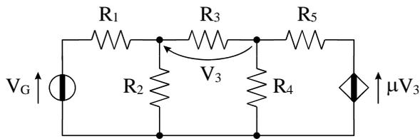
$$\begin{aligned} R_1 &= 5 \, \Omega \\ R_2 &= 5 \, \Omega \\ R_3 &= 2 \, \Omega \\ R_4 &= 2 \, \Omega \\ R_5 &= 10 \, \Omega \\ V_G &= 30 \, \text{V} \\ \mu &= 4 \end{aligned}$$
