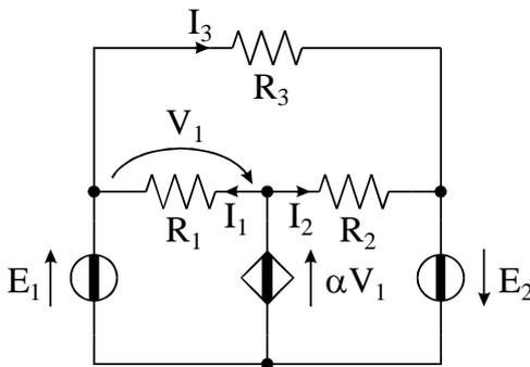
$$\begin{aligned} R_1 &= 4 \, \Omega \\ R_2 &= 10 \, \Omega \\ R_3 &= 4 \, \Omega \\ E_1 &= 8 \, \text{V} \\ E_2 &= 8 \, \text{V} \\ \alpha &= 3 \end{aligned}$$
