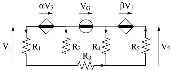
$$\begin{aligned} R_1 &= 6 \, \Omega \\ R_2 &= 2 \, \Omega \\ R_3 &= 2 \, \Omega \\ R_4 &= 6 \, \Omega \\ R_5 &= 2 \, \Omega \\ V_G &= 16 \, \text{V} \\ \alpha &= 1/2 \\ \beta &= 1/3 \end{aligned}$$
