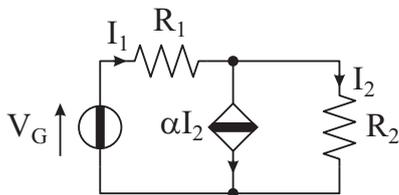
$$\begin{aligned} R_1 &= 3 \, \Omega \\ R_2 &= 3 \, \Omega \\ V_G &= 15 \, \text{V} \\ \alpha &= 3 \end{aligned}$$
