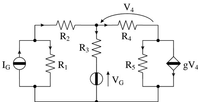
$$\begin{aligned} R_1 &= 6 \Omega \\ R_2 &= 3 \Omega \\ R_3 &= 3 \Omega \\ R_4 &= 3 \Omega \\ R_5 &= 6 \Omega \\ g &= 0.25 \text{ S} \\ I_G &= 6 \text{ A} \\ V_G &= 24 \text{ V} \end{aligned}$$
