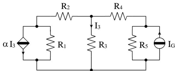
$$\begin{aligned} R_1 &= 3 \, \Omega \\ R_2 &= 6 \, \Omega \\ R_3 &= 6 \, \Omega \\ R_4 &= 3 \, \Omega \\ R_5 &= 5 \, \Omega \\ I_G &= 6 \, \text{A} \\ \alpha &= 4 \end{aligned}$$
