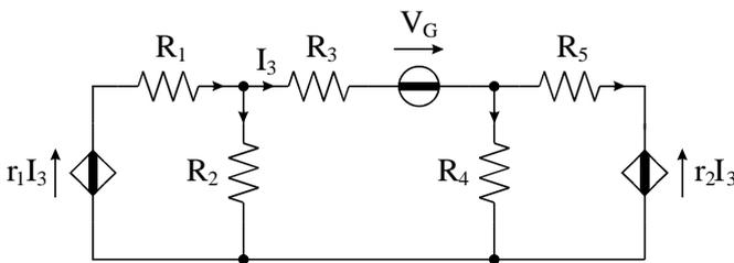
$$\begin{aligned} R_1 &= 2 \Omega \\ R_2 &= 10 \Omega \\ R_3 &= 4 \Omega \\ R_4 &= 8 \Omega \\ R_5 &= 4 \Omega \\ r_1 &= 8 \Omega \\ r_2 &= 2 \Omega \\ V_G &= 12 \text{ V} \end{aligned}$$
