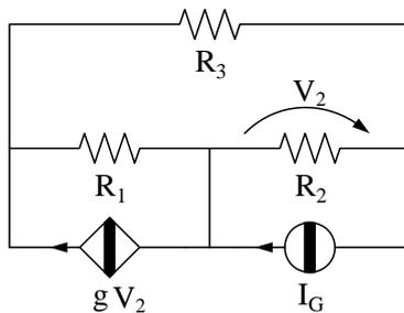
$$\begin{aligned} R_1 &= 1 \, \Omega \\ R_2 &= 3 \, \Omega \\ R_3 &= 2 \, \Omega \\ I_G &= 3 \, \text{A} \\ g &= 0.5 \, \text{S} \end{aligned}$$
