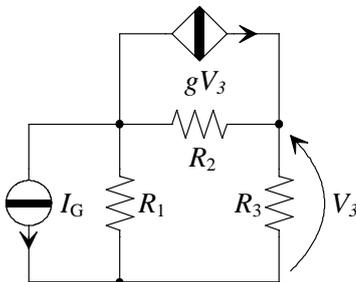
$$\begin{aligned} R_1 &= 2 \, \Omega \\ R_2 &= 4 \, \Omega \\ R_3 &= 2 \, \Omega \\ I_G &= 4 \, \text{A} \\ g &= 2 \, \text{S} \end{aligned}$$
