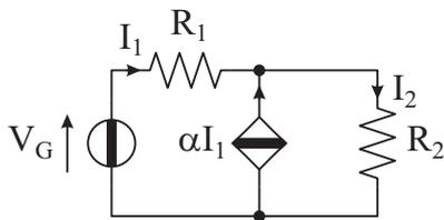
$$\begin{aligned} R_1 &= 4 \, \Omega \\ R_2 &= 2 \, \Omega \\ V_G &= 12 \, \text{V} \\ \alpha &= 3 \end{aligned}$$
