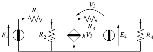
$$\begin{aligned} R_1 &= 4 \, \Omega \\ R_2 &= 2 \, \Omega \\ R_3 &= 4 \, \Omega \\ R_4 &= 6 \, \Omega \\ E_1 &= 12 \, \text{V} \\ E_2 &= 12 \, \text{V} \\ g &= 0.5 \, \text{S} \end{aligned}$$
