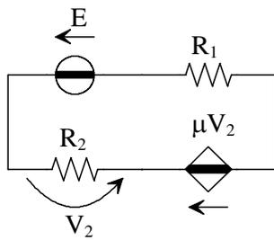
$$\begin{aligned} R_1 &= 4 \, \Omega \\ R_2 &= 2 \, \Omega \\ E &= 12 \, \text{V} \\ \mu &= 5 \end{aligned}$$
