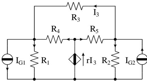
$$\begin{aligned} R_1 &= 3 \Omega \\ R_2 &= 3 \Omega \\ R_3 &= 3 \Omega \\ R_4 &= 3 \Omega \\ R_5 &= 3 \Omega \\ I_{G1} &= 3 \text{ V} \\ I_{G2} &= 9 \text{ V} \\ r &= 2 \Omega \end{aligned}$$
