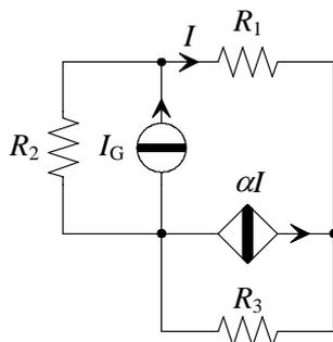
$$\begin{aligned} R_1 &= 4 \, \Omega \\ R_2 &= 3 \, \Omega \\ R_3 &= 1 \, \Omega \\ I_G &= 4 \, \text{A} \\ \alpha &= 4 \end{aligned}$$
