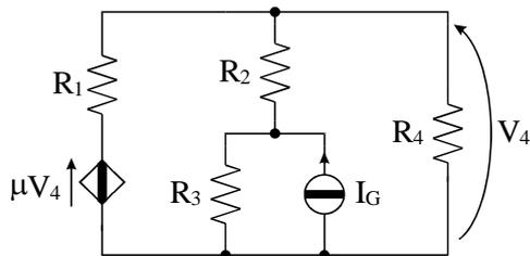
$$\begin{aligned} R_1 &= 8 \, \Omega \\ R_2 &= 4 \, \Omega \\ R_3 &= 4 \, \Omega \\ R_4 &= 8 \, \Omega \\ I_G &= 6 \, \text{A} \\ \mu &= 6 \end{aligned}$$
