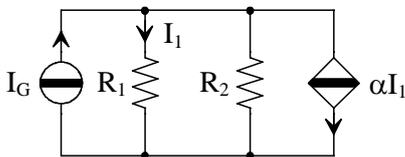
$$\begin{aligned} R_1 &= 4 \, \Omega \\ R_2 &= 2 \, \Omega \\ I_G &= 5 \, \text{A} \\ \alpha &= 2 \end{aligned}$$
