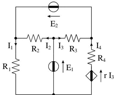
$$\begin{aligned} R_1 &= 3 \Omega \\ R_2 &= 3 \Omega \\ R_3 &= 3 \Omega \\ R_4 &= 3 \Omega \\ E_1 &= 9 \text{ V} \\ E_2 &= 12 \text{ V} \\ r &= 2 \Omega \end{aligned}$$
