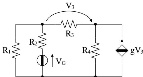
$$\begin{aligned} R_1 &= 4 \, \Omega \\ R_2 &= 4 \, \Omega \\ R_3 &= 2 \, \Omega \\ R_4 &= 2 \, \Omega \\ V_G &= 12 \, \text{V} \\ g &= 3 \, \text{S} \end{aligned}$$
