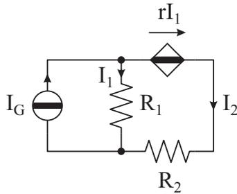
$$\begin{aligned} R_1 &= 4 \, \Omega \\ R_2 &= 4 \, \Omega \\ I_G &= 5 \, \text{A} \\ r &= 2 \, \Omega \end{aligned}$$
