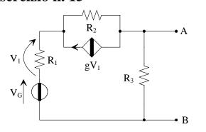
$$\begin{aligned} R_1 &= R \\ R_2 &= R_3 = 2R \end{aligned}$$
