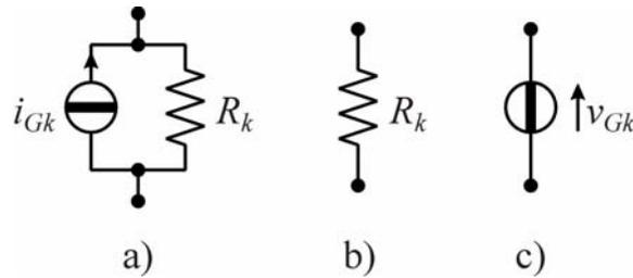
$$i_{eq} = \frac{\sum_{k \in \mathcal{A}} R_k i_{Gk} + \sum_{k \in \mathcal{C}} v_{Gk}}{\sum_{k \in \mathcal{A} \cup \mathcal{B}} R_k} \qquad R_{eq} = \sum_{k \in \mathcal{A} \cup \mathcal{B}} R_k$$
