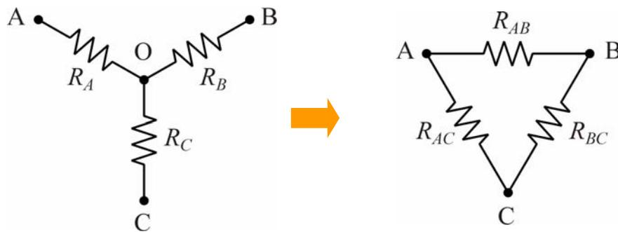
$$R_{AB} = \frac{R_A R_B + R_A R_C + R_B R_C}{R_C}$$
