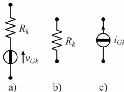
$$v_{eq} = \frac{\sum_{k \in \mathcal{A}} G_k v_{Gk} + \sum_{k \in \mathcal{C}} i_{Gk}}{\sum_{k \in \mathcal{A} \cup \mathcal{B}} G_k}$$
