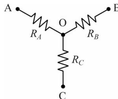
$$R_A = \frac{R_{AB} R_{AC}}{R_{AB} + R_{AC} + R_{BC}}$$
