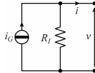
$$i = i_G - \frac{v}{R_I} \Rightarrow v = R_I i_G - R_I i$$
