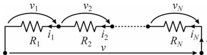
$$i = \frac{v}{R_S} = \frac{v}{\sum_{k=1}^N R_k} \quad \Rightarrow \quad v_j = R_j i = \frac{R_j}{\sum_{k=1}^N R_k} v \quad (j = 1, \dots, N)$$
