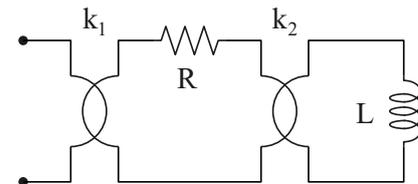
$R = 100 \ \Omega \quad L = 2 \text{ mH} \quad \omega = 1000 \text{ rad/s}$
