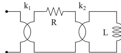
$R = 18 \Omega \quad L = 2 \text{ mH} \quad \omega = 1000 \text{ rad/s}$
