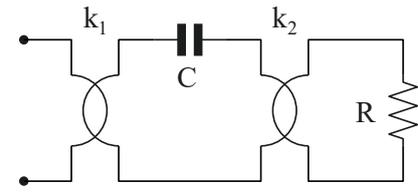
$R = 10 \Omega$     $C = 25 \mu\text{F}$     $\omega = 1000 \text{ rad/s}$
