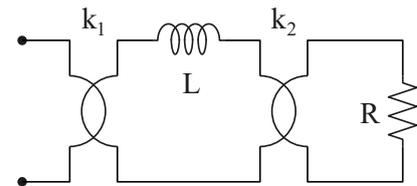
$R = 2 \Omega \quad L = 50 \text{ mH} \quad \omega = 1000 \text{ rad/s}$
