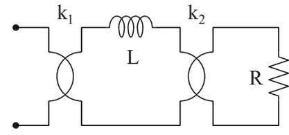
$R = 5 \Omega \quad L = 45 \text{ mH} \quad \omega = 1000 \text{ rad/s}$
