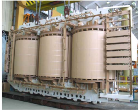
ConventioneI 400 MVA Transformer
