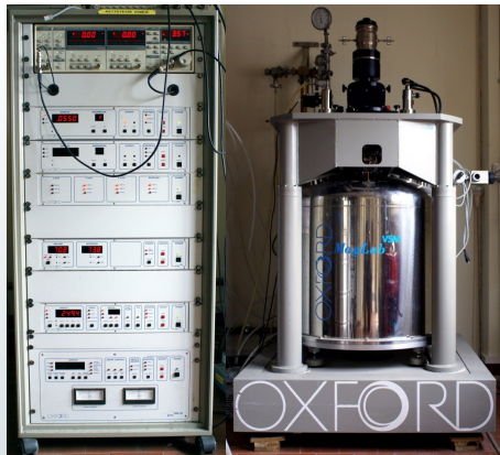
— VSM system at ENEA —
