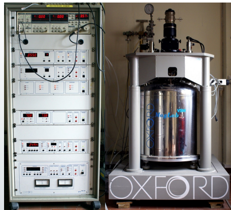
— VSM system at ENEA —
