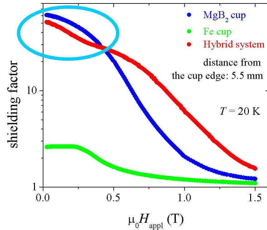
Shielding factor of the hybrid system: **no straightforward composition of the independent contributions** of the two shields:
