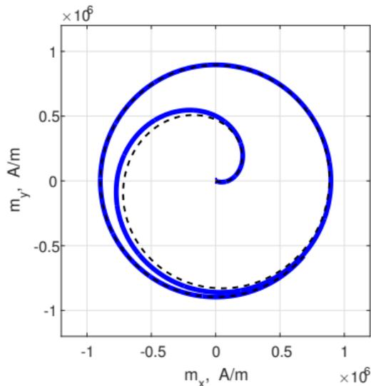
The model solution  $\mathbf{m} = (m_x, m_y)$  (solid line) and the one based on the explicit approximation (dashed line) are close in this case.
