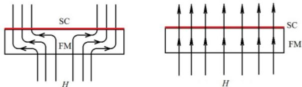
Fig:  $\mathbf{b}$  lines for a weak (left) and strong (right) external field.
