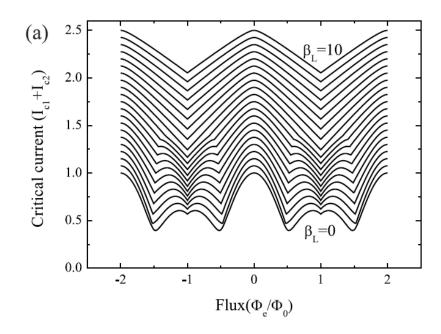
The increase of the  $\sin(\phi/2)$  component causes a decrease of the oscillation amplitude without introducing a  $2\Phi_0$  component.
