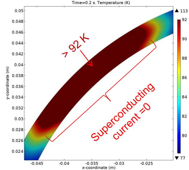
Field "cut-off" is well after end of heat pulse
