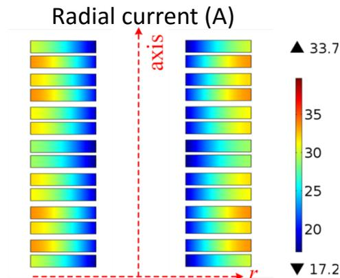
Charging in a intra- & inter-coil graded magnet
