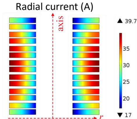
Charging in a inter-coil graded magnet
