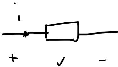
$$P = \frac{1}{T} \int_0^T p(t) dt = V_e I_e \cos \varphi \quad (\text{W})$$
