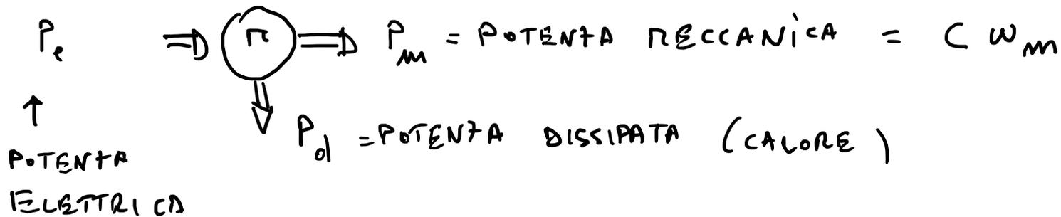
$$\eta = \text{RENDIMENTO} = \frac{P_m}{P_e} = \frac{\Delta E_m}{\Delta E_e} \approx \frac{\langle P_m \rangle (t_2 - t_1)}{\langle P_e \rangle (t_2 - t_1)}$$
